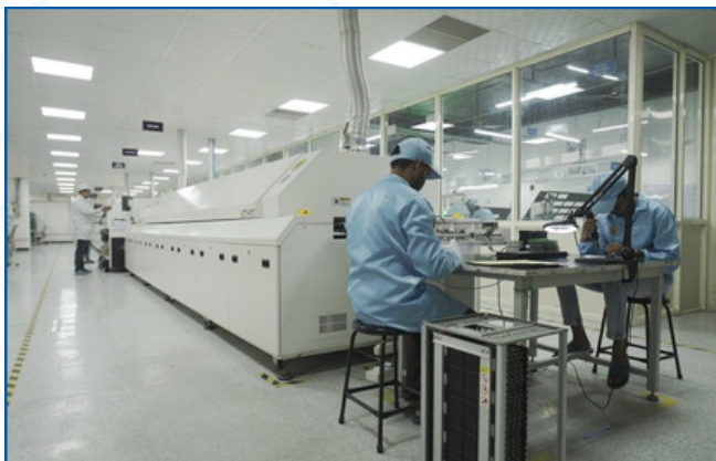
Reflow line and inspection bay
